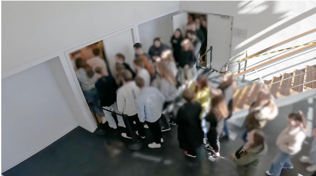
Figure 4 - Experiment on the throughput of a door
